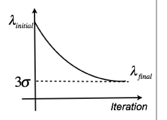
High initial thresholds to extract the most significant features. Then, the thresholds decrease to retrieve more detailed information about the sources.
